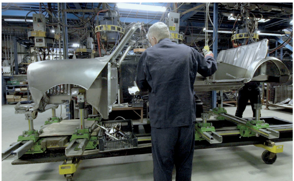
ABOVE & BELOW Here we see the production of the Mini's seam-welded Heritage bodysell in progress. Common sense suggests new metal is preferable to old when it comes to racing
