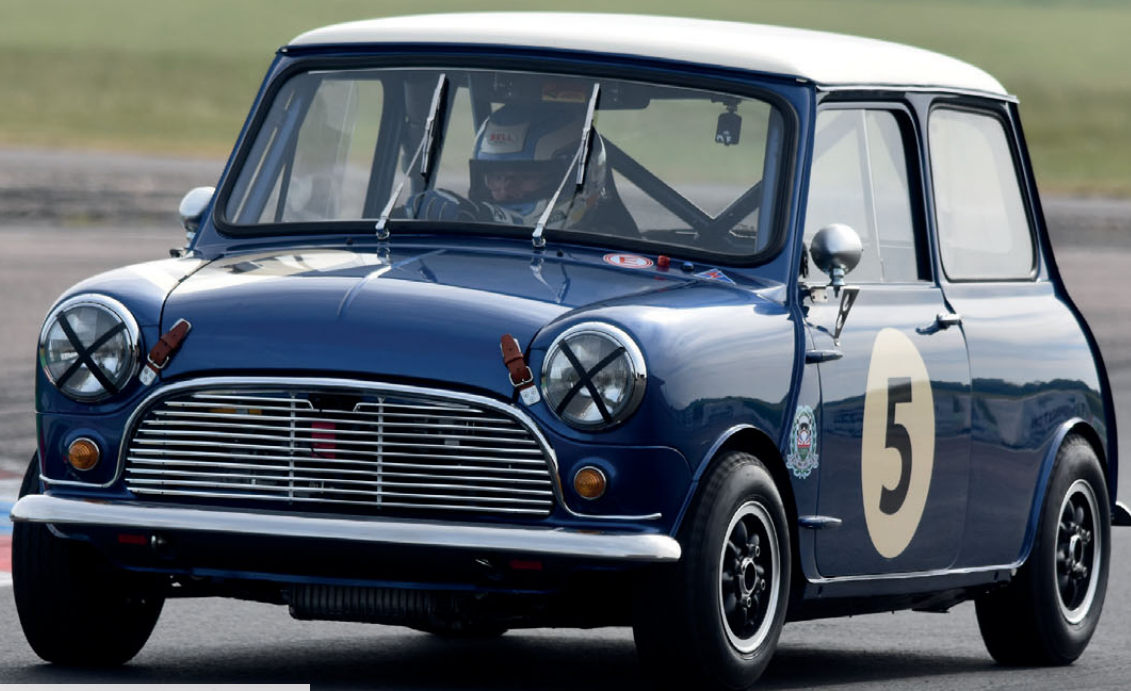
ABOVE The team's Mini is brimming with off-the-shelf BMH parts, including seam-welded Heritage bodyshell, Heritage subframes, and alloy door and boot skins
